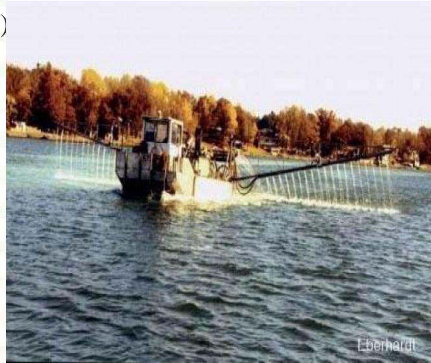
Figure 6 Phosphorus inactivation by alum treatment.
